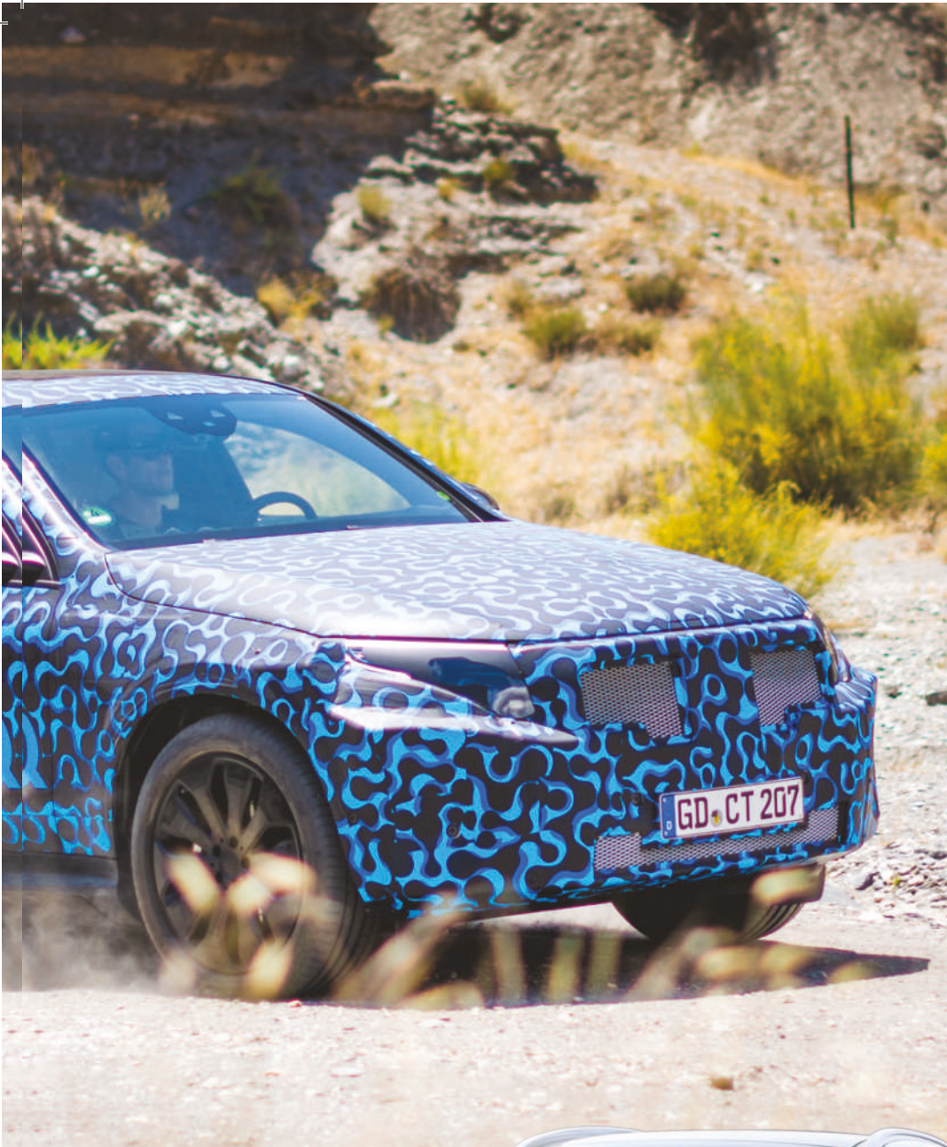
2&3. The Mercedes-Benz GLC F-Cell is powered by a new fuel cell/electric hybrid powertrain, but uses a tried and tested vehicle architecture
