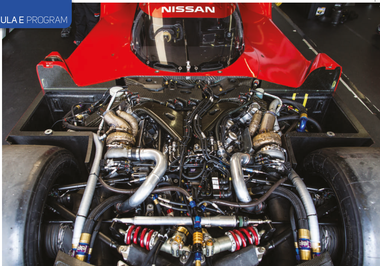
The drive system in the GT-R LM comprised a twin-turbocharged 3.0-liter V6 petrol engine and a mechanical flywheel KERS
