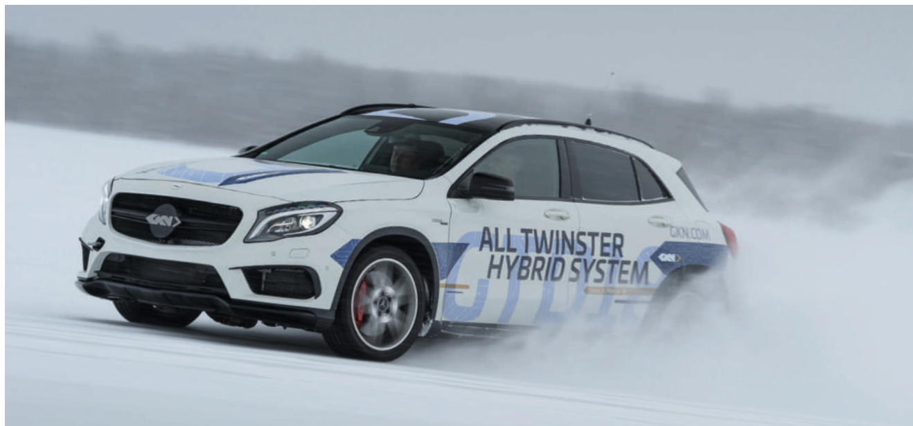
The testbed for eTwinsterX is GKN's Mercedes-AMG GLA 45 prototype vehicle. The car was reengineered by GKN for use at its cold-weather testing facility in Arjeplog, Sweden
