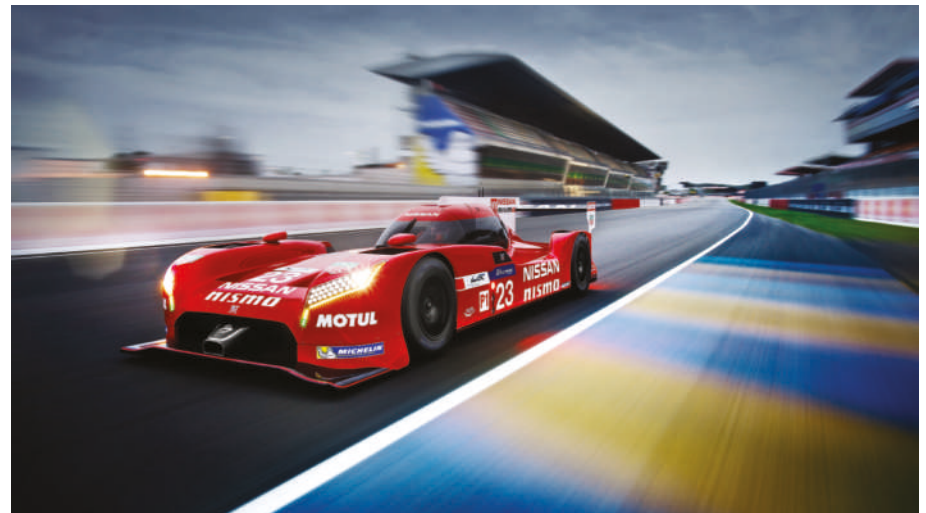
Left and below: In 2015, Nissan's LMP1 entry raced Le Mans without its hybrid system engaged after it was found that the GT-R LM gained no benefit from hybrid power
