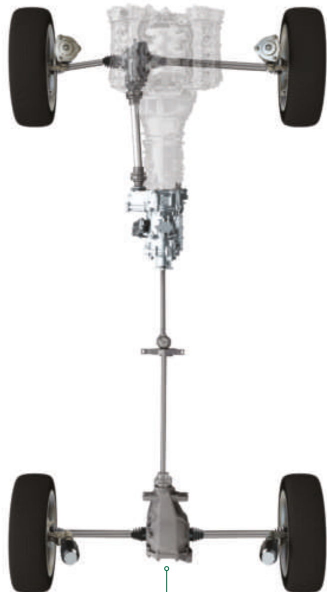
The layout of Magna Powertrain's 48V transfer case in the vehicle drivetrain
