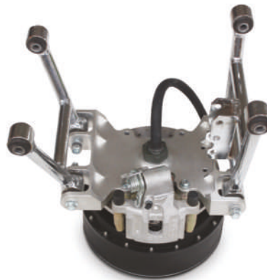
The Luka EV uses four 12.5kW in-wheel motors
