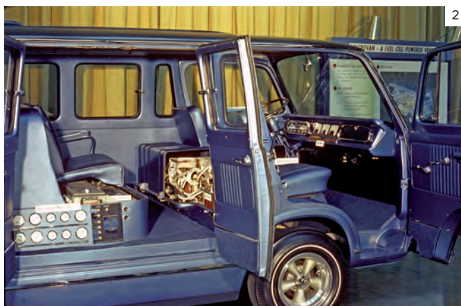
1. The GM Electrovan featured 32 series-connected fuel cells providing 540V DC
