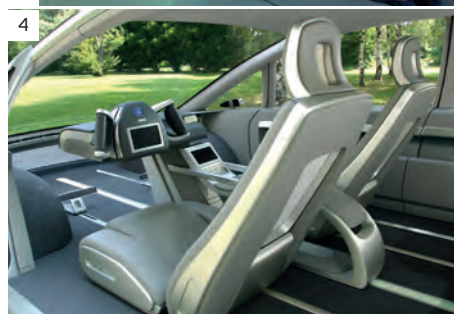
4. The Hy-Wire was powered by fuel cell technology and hub motors, free of ICE packaging constraints
