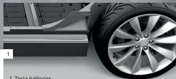
1. Tesla batteries feature upright cylindrical cells spread out across the vehicle floor
