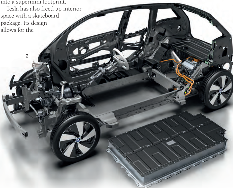
2. The 'Life' cabin of the BMW i3 sits on top of the 'Drive' chassis, increasing vehicle interior space
