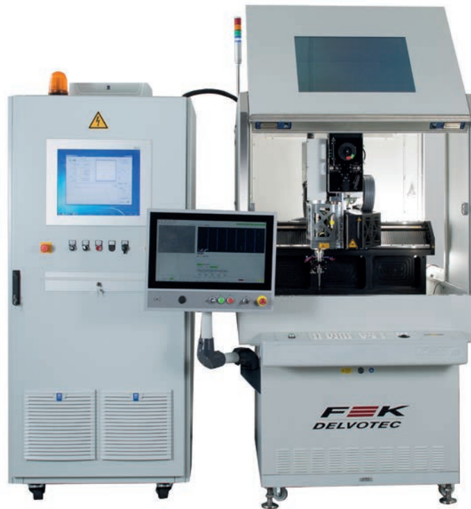
The Laserbonder contains a wirebonder base with large working area (right) and a standard fiber laser with a control unit (left). Parts handling can be automated in a variety of ways, from manual loading and unloading to full in-line capability
