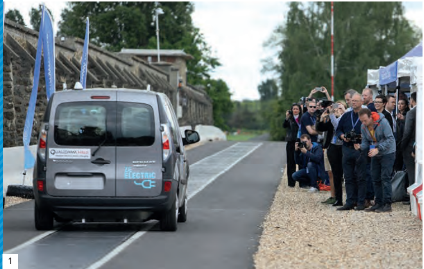
1. Dynamic charging demonstrations took place at a 100m-long test track built at Satory Versailles
