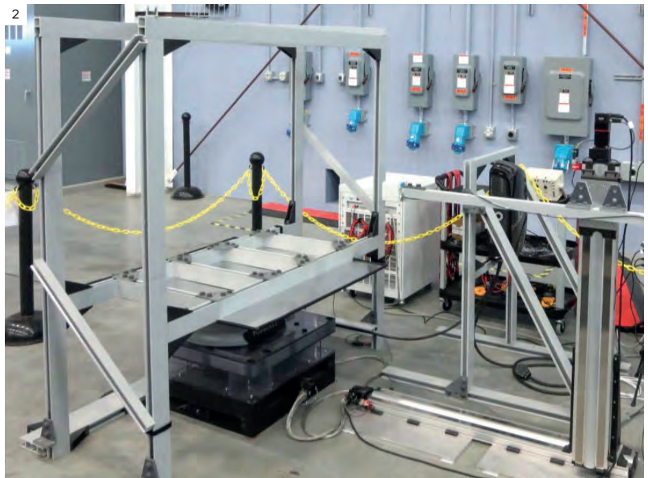
2. Idaho National Laboratory researchers and six companies achieved a major milestone in December 2016 by completing bench testing for wireless charging systems, a technology that eliminates the need to plug in electrified vehicles
