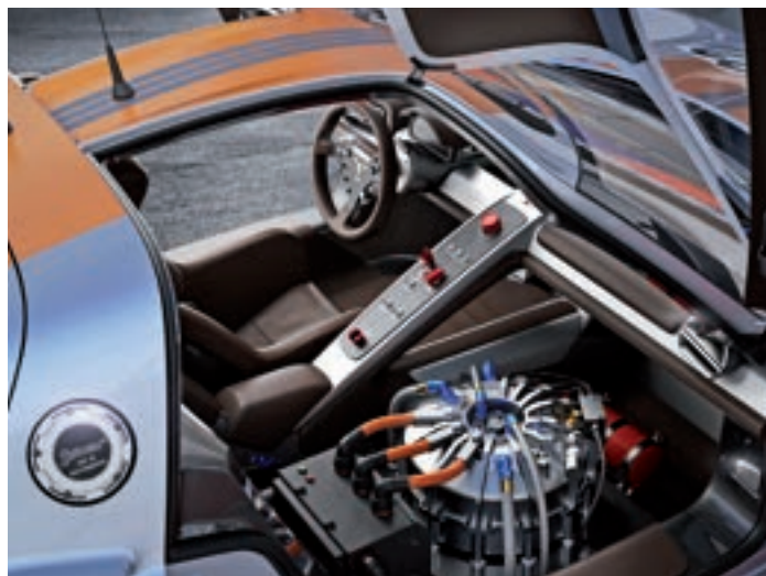
Above and right: At the 2011 Detroit Motor Show, Porsche unveiled the RSR racing variant of the then 918 Spyder concept. Instead of using plug-in hybrid technology, power for the two electric motors is provided by a flywheel accumulator KERS system that sits beside the driver in the passenger compartment
