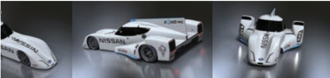
3. The narrow front track and wide rear design mean the car is not only much lighter than a conventional square construction, but it also creates a lot less drag
