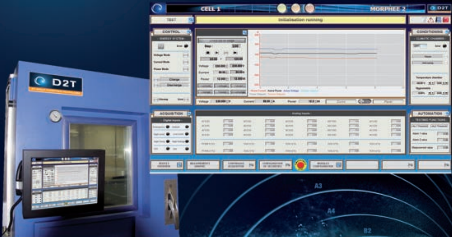
Component test bed for battery application
