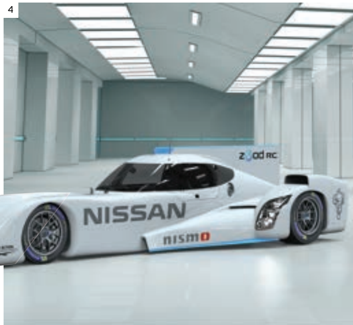
3. The narrow front track and wide rear design mean the car is not only much lighter than a conventional square construction, but it also creates a lot less drag
