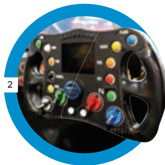
2. An aircraft-type steering wheel and state-of-the-art instrumentation complement the glider-like experience of the zero-emissions prototype racer
