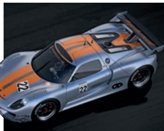
Above and right: At the 2011 Detroit Motor Show, Porsche unveiled the RSR racing variant of the then 918 Spyder concept. Instead of using plug-in hybrid technology, power for the two electric motors is provided by a flywheel accumulator KERS system that sits beside the driver in the passenger compartment
