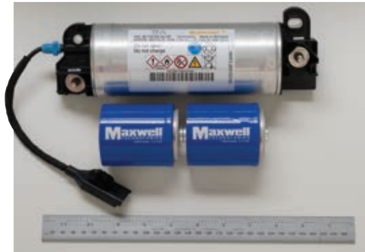
Automotive engineers at Continental have created a highly acclaimed energy storage device that makes use of Maxwell ultracapacitors
