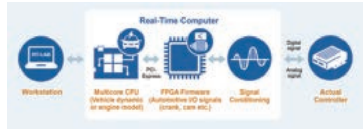
The architecture of the FPGA-based simulation testing used by OPAL-RT
