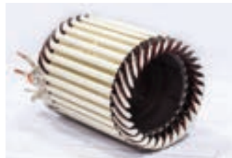
An external rotor and internal stator machine has a longer radius than other topologies, generating more torque while using less material
