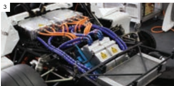
3. Featuring two axial flux electric motors and a 42kWh lithium-ceramic battery, the TMG EV P002 tops out at 230km/h, with a maximum power output of 543ps at 6,000rpm and 1,200Nm of peak torque
