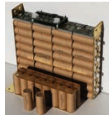
The lithium-iron-phosphate cylindric cells used inside Paragon's F-Power battery system boast higher efficiency
