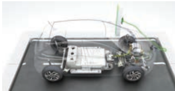
The Renault Zoe has a 22kWh lithium-ion battery that delivers a driving range of 210km under the NEDC cycle. But will this technology soon be surpassed by an advanced sulfur-based chemistry?
