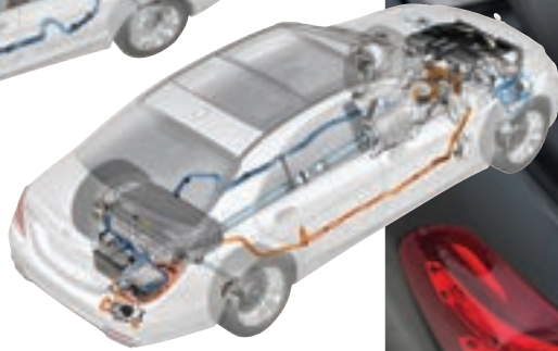
2. An externally rechargeable battery pack results in around 30km of emissions-free driving
