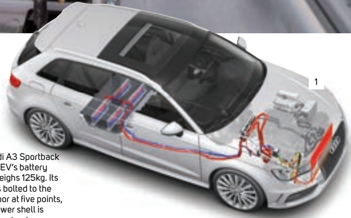
2. The Sportback e-tron's battery module consists of 96 prismatic cells arranged into eight modules of 12 cells
