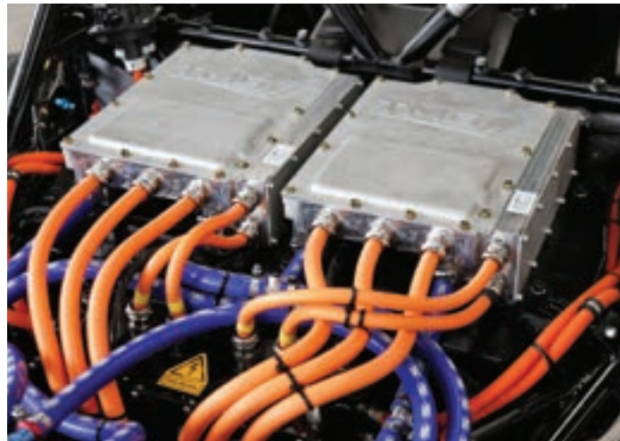
TMG specializes in the integration and development of EV powertrains, such as with this 400kW example
